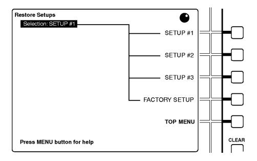
Figure 31: The Restore Setups submenu
